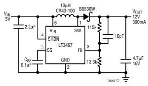
Figure 5.  $5V_{IN}$  to 12V at 300mA BOOST Converter
