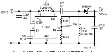
Figure 1.  $10V_{IN}$ - $16V_{IN}$  to 12V at 300mA SEPIC Converter
