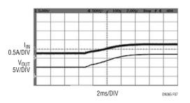
Figure 7. Input Current and Output Voltage at Turn-On with  $\mathsf{C}_{SS}$  Capacitor for Figure 5 Circuit
