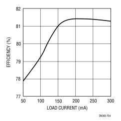
Figure 4. SEPIC Converter Efficiency for Figure 1 Circuit
