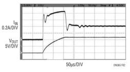
Figure 2. Input Current and Output Voltage at Turn-On Without  $\mbox{C}_{SS}$  Capacitor for Figure 1 Circuit
